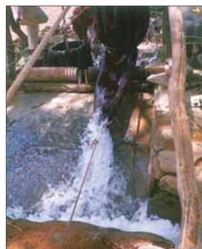
Figure 11. A traditional water lifting device (Chadas) used for irrigation before watershed program, Gokulpura-Goverdhanpura watershed.
