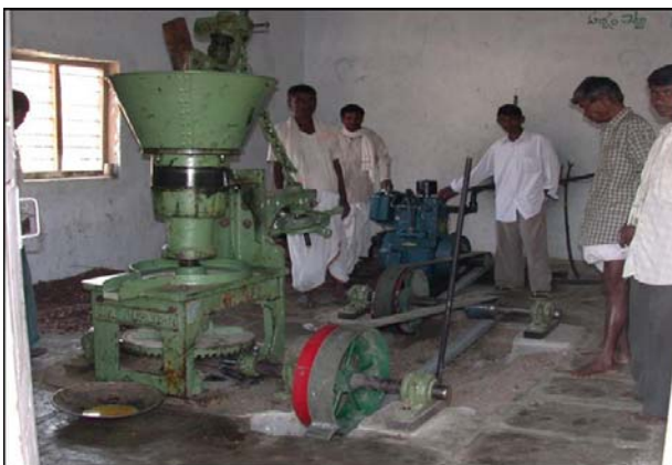
Figure 3. Pongamia seed oil extraction unit in Powerguda.
